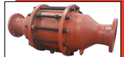
A flame arrester is designed to be used as a barrier between the tank and the vent to safeguard the tank contents from igniting if an outside ignition source is present. A detonation arrester isolates the potential ignition of vapors in closed piping systems to protect storage tanks and process units from detonation flame fronts.
