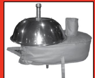
Shand & Jurs insulation jackets provide heat retention for equipment in cold weather environments. Construction of the insulating jacket is silicone impregnated woven glass cloth lining with 1" thick fiber glass material. The jacket is easy to install and remove in the field.
